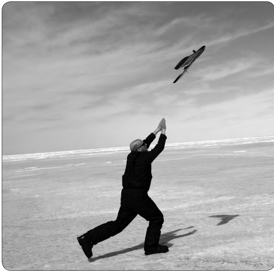
Dr. Paul Cooley launches a drone to study the ice on Lake Winnipeg. Images from the drone were checked against satellite data to determine ice conditions.
